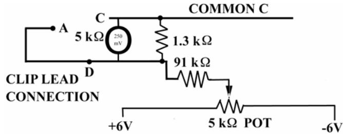
**Figure 8: Calibration Circuit**
