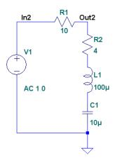
The impedance of the resistor is  $Z_R = R$  (constant for all frequencies) and the impedance of the inductor is  $Z_L = i\omega L$ .
