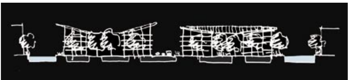
figure 7: cross section showing sequence of transformed city block pattern, every third canal remains for rain and gray water (proposed)
