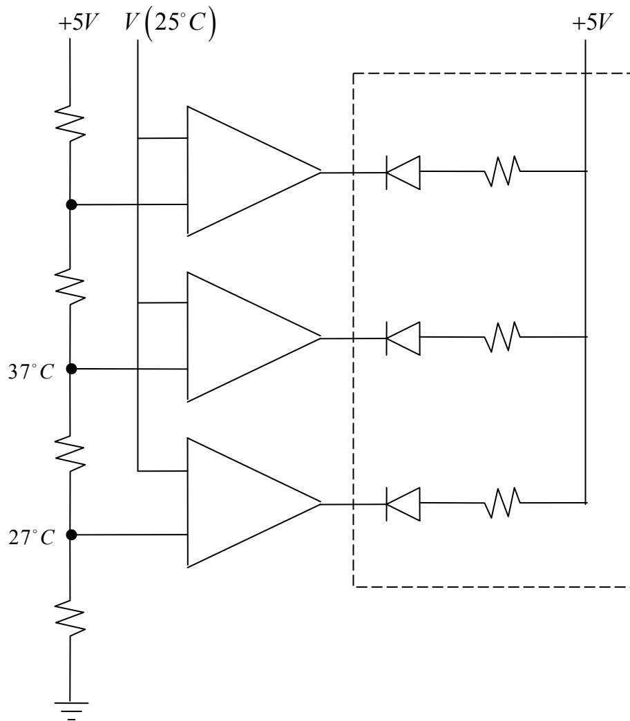
Connect the input of a series of op-amps in such a way that there is a common voltage ( $V_{\text{TERM}}$ ) reaching the inputs of all op amps. Choose resistor values to create reference voltages that represent different temperature values. Since the 555 is better at sinking current rather than sourcing it, connect LEDs as shown above.
