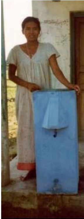
Fig 2. An existing Biosand filter in Nepal
