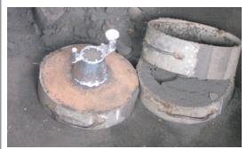
A cast corn sheller with sprues attached.
