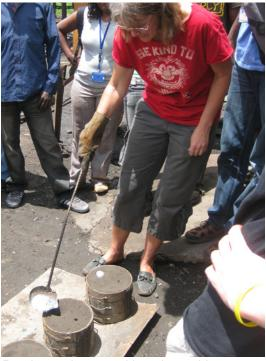
Pouring molten metal into the molds.
