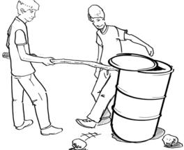
Carefully remove the stones from under the drum while supporting the drum with a stick.
