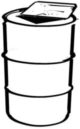
A piece of sheet metal is needed to cover the top hole and prevent oxygen from entering the drum, allowing the material inside to carbonize.
