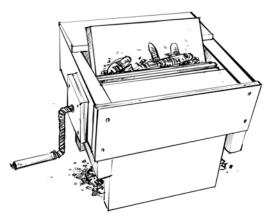
A charcoal crushing machine can be used for large quantities.
