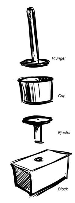
Fig 1 The four components of the \$2 charcoal press
