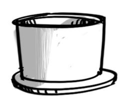
Fig 2b Overhang endplate configuration
