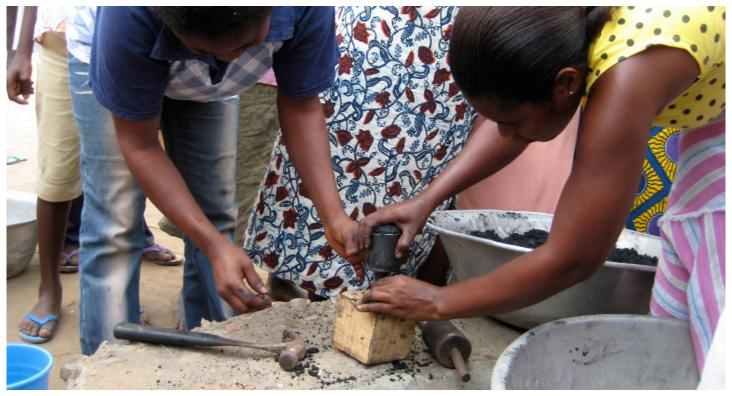
This project is a very low-cost device for forming charcoal briquettes. It is composed of three welded metal parts and a wooden block. To make it, you will learn to use a band saw, a sander, a drill press, the OMAX water jet cutter and several hand tools. You will also learn to do some basic welding.
