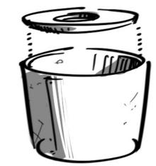
Fig 2a Press fit an endplate configuration
