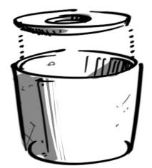
Fig 2a Press fit an endplate configuration
