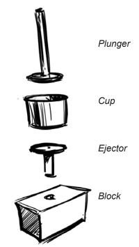
Fig 1 The four components of the \$2 charcoal press
