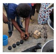
6. Pressing charcoal mixture into briquettes
