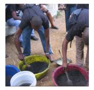
5. Mixing binder, water and charcoal to make briquettes
