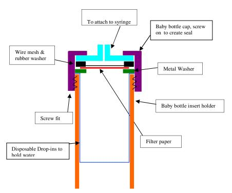
Design Schematic of Test Water Cheap Filter Holder
