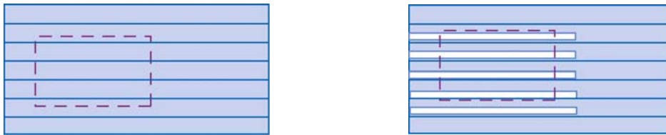
Figure 10.5.3 Eddy currents can be reduced by (a) laminating the slab, or (b) making cuts on the slab.
