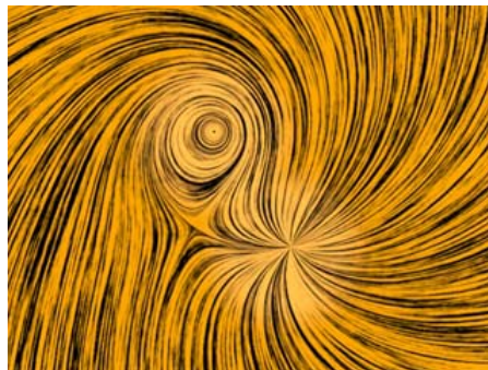
Figure 1.4.8 A flow field that has both a source (divergence) and a circulation (curl).
