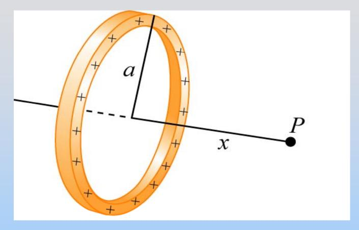
P on axis of ring of charge, x from center Radius a, charge density  $\lambda$ .
