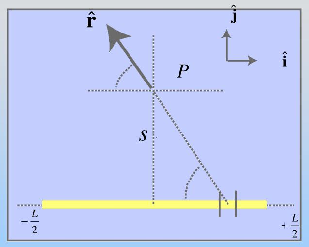
Point *P* lies on perpendicular bisector of uniformly charged line of length *L*, a distance *s* away. The charge on the line is *Q*. What is *E* at *P*?
