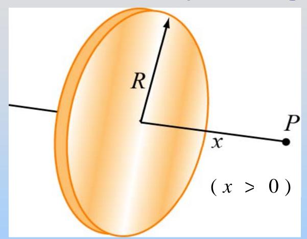
P on axis of disk of charge, x from center Radius R, charge density  $\sigma$ .
