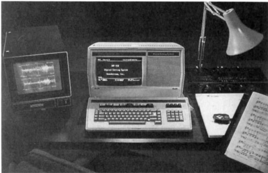
Figure 16.38 The Soundstream editing system, ca. 1982. The console in the center was used to enter editing commands. The monitor at the left displayed time-domain waveform images.
