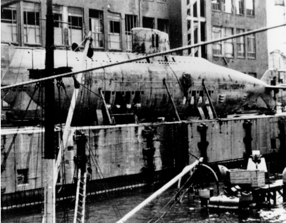
Walter Type XVIIIB up on the stocks. Pictured above is the German Walter Type XVIIIB U-1406 , partially dismantled shortly after the end of World War II. U-1406 was turned over to the U.S. Navy as a war prize and soon disposed of, but the Royal Navy later operated her sister ship, U-1407 , as HMS Meteorite to gain experience in hydrogen-peroxide propulsion technologies.
