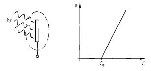
Figure 3.7: Photo-electric effect: (a) Schematic setup and (b) dependence of the necessary grid voltage to supress the electron current as a funtion of light frequency.
