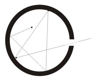
Figure 3.1: The Ulbricht sphere, is a sphere with a small opening, where only a small amount of radiation can escape, so that the interior of the sphere is in thermal equilibrum with the walls, which are kept at a constant tremperature. The inside walls are typically made of diffuse material, so that after multiple scattering of the walls any incoming ray is absorbed, i.e. the wall opening is black.
