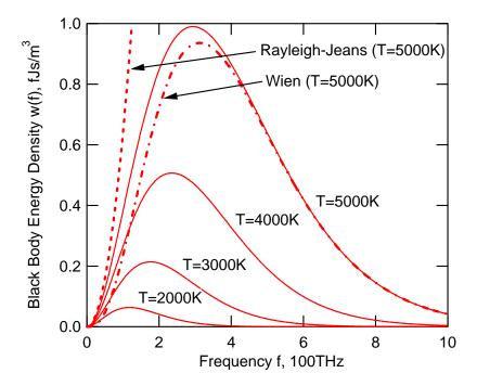
Figure 3.2: Spectral energy density of the black body radiation according to Planck's Law.
