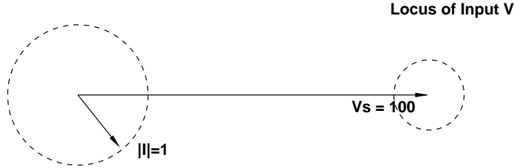
Figure 3: Locus of Current and Voltage Phasors
