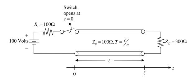
A transmission line of length  $\ell$ , characteristic impedance  $Z_0 = 100\Omega$ , and one-way time of flight  $T = \frac{\ell}{c}$  is connected at z = 0 to a 100 volt DC battery through a series source resistance  $R_s = 100\Omega$  and a switch. The  $z = \ell$  end is loaded by a 300 $\Omega$  resistor.
