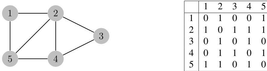
Figure 1: Adjacency matrix representation of an undirected graph.
