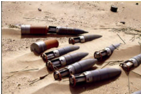
Figure 11. The effects of high temperatures exacerbate the risk of accidental detonation of abandoned ammunition. These items were found in the Kuwaiti desert where they had lain in the sun for several months (photo by the author 1991)
