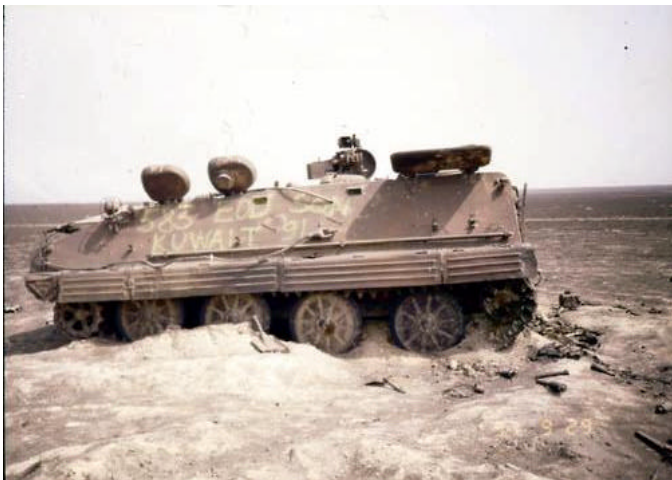
Figure 31. EOD teams may be used to respond to more complicated tasks than conventional mine clearance. For example, clearing abandoned armoured vehicles (above) or abandoned ammunition stockpiles (right). Note that the EOD team has marked this vehicle to show it has been cleared.
