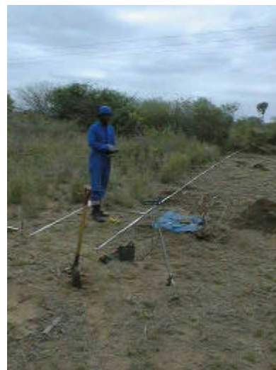
Figure 24. The systematic approach to demining can be seen in this photograph of a deminer preparing to start work in Mozambique. The wooden stick next to the deminer's left foot is the base line that marks the forward edge of the cleared area. The area to the front of the deminer has already been cleared (as can be seen from the shorter vegetation). The deminer's protective equipment and mine detector are laid out in the cleared area (photo by the author, 1997)
