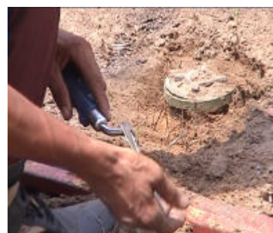
Figure 26. The demining cycle in Cambodia. In the first picture, the deminer searches the ground immediately to the front of the baseline with his mine detector (this team uses a second stick to mark the forward edge of the search area). In the second photograph the deminer uses a prodder to investigate a detector signal by probing for a possible buried mine (the prodder is just visible under his left hand). In the third photograph the deminer has found and excavated the mine using a trowel (photos by the author, 1998).
