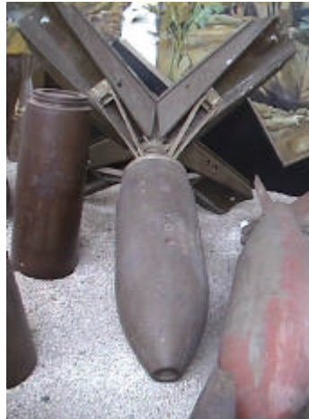
Figure 7. A selection of aircraft bomb casings kept in a museum in Vietnam. The large tail fins at the rear of the bomb in the centre are designed to slow down the bomb so that it explodes behind the low-flying aircraft that drops it (photo by the author 2000)
