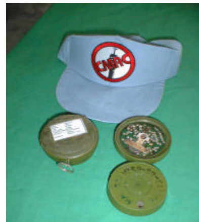
Figure A-3. This Chinese AP mine includes an electronic anti-handling device (photo by the author, Cambodia 1998)
