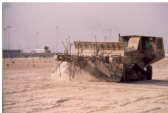
Figure 36. A flail machine being used in Kuwait. Note the chains rotating around the central drum and the use of a protective shield between the flail and the rest of the vehicle (photo by the author, 1991).
