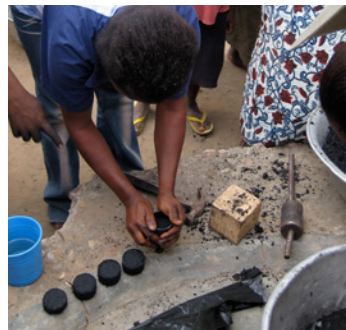
6. Pressing charcoal mixture into briquettes
