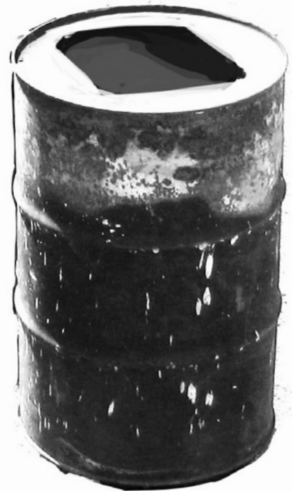
Charcoal Drum ($15) – converts agricultural waste into carbonized material for charcoal in a couple hours
