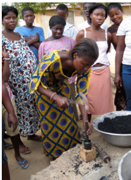
Third Prototype $2 10-12 Briquettes a Minute
