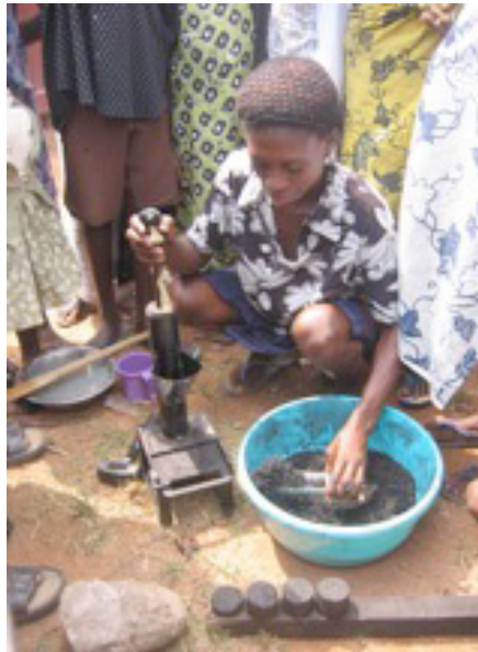
Second Prototype $20 6-8 Briquettes a Minute
