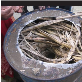
1. Placing bagasse in the oil drum
