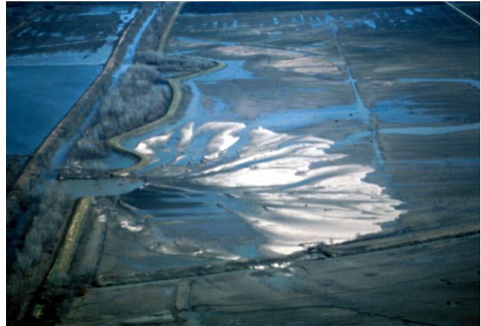
Crevasse splay sand from levee break at Bryants Creek MO crossing floodplain of upper Mississippi River near mile 260. Photo by R.H. Meade, USGS
