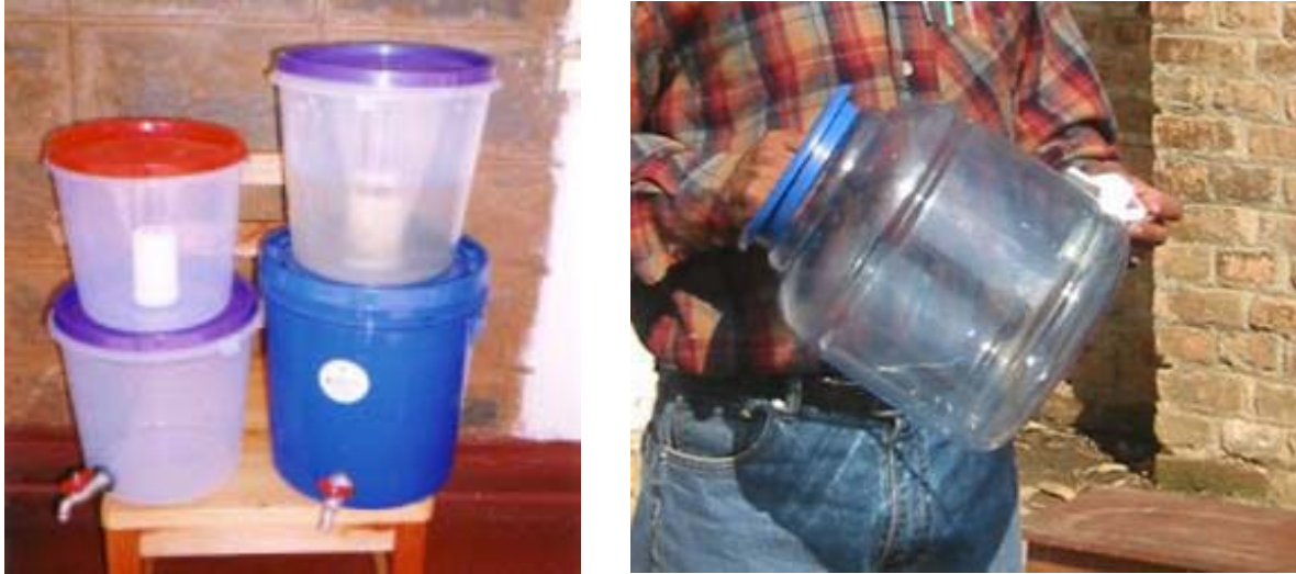
Figure 16: Examples of Filter Systems and Containers that use Clear Plastic: Kisii Filter System, Kenya (left); Durable Plastic Container (right).
