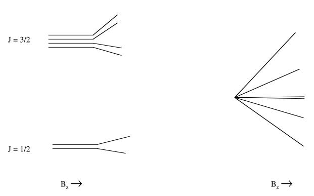
Note that every eigenstate has a different Zeeman tuning rate. The gross energy level pattern and the Zeeman tuning rates tell which limiting case one is near and which state is which. The details of the nonlinear Zeeman tuning of one *assigned* level determine  $\zeta$  and  $\gamma$ .
