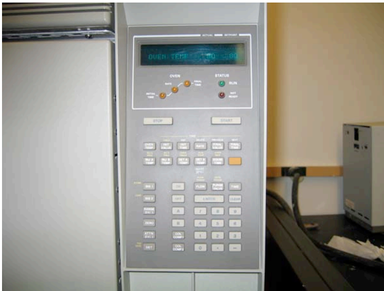
Figure 9. Keyboard of GC HP-5890A.
