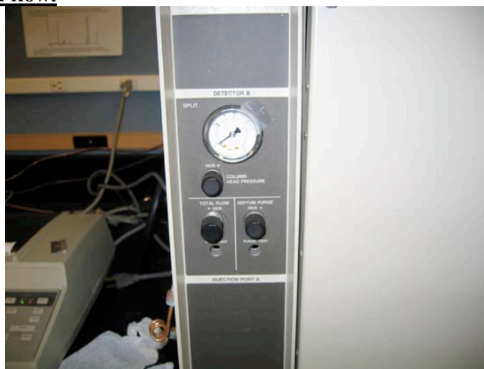
Figure 10. Column head pressure gauge (should read 16 psi).
