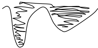
Figure 4. The molecule is heated and then cooled slowly so that conformational changes taking place will lead to a local minimum. This process is repeated many times until several closely related, low energy, conformations are obtained.
