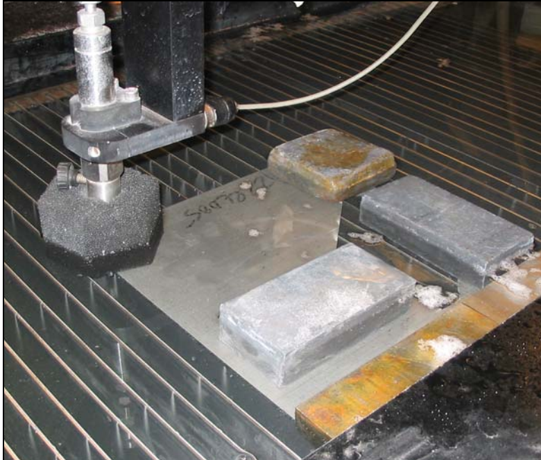
Figure 45 Water level raised - ready to begin machining
