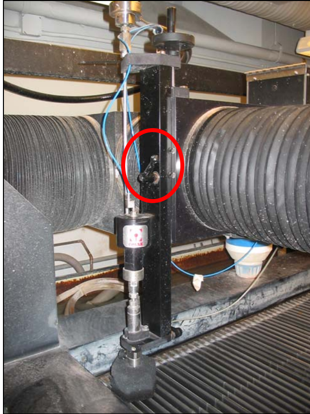
Figure 44 Location of lever to lock-in desired height of water jet cutter nozzle
