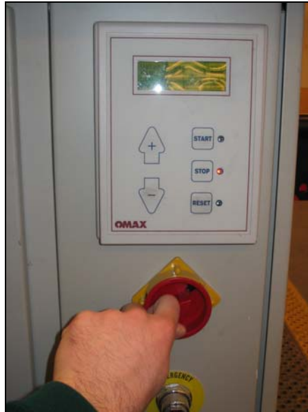
Figure 35 Turning on/off power to water jet cutter
