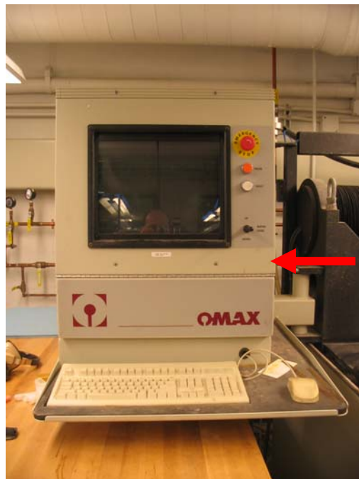
Figure 34 Location of power switch to water jet system
