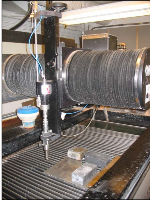
Figure 40 Setup of part to cut with water jet cutter
