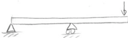
Pinned, simply supported
