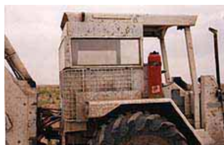
Fig. 3: Polycarbonate Windows on a Armoured Backhoe Cab
