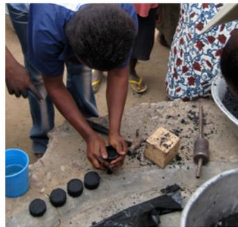
6. Pressing charcoal mixture into briquettes
