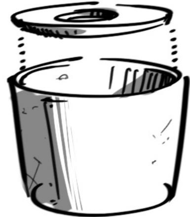
Fig 2a Press fit an endplate configuration
