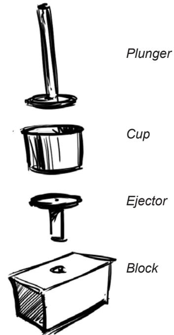
Fig 1 The four components of the \$2 charcoal press
