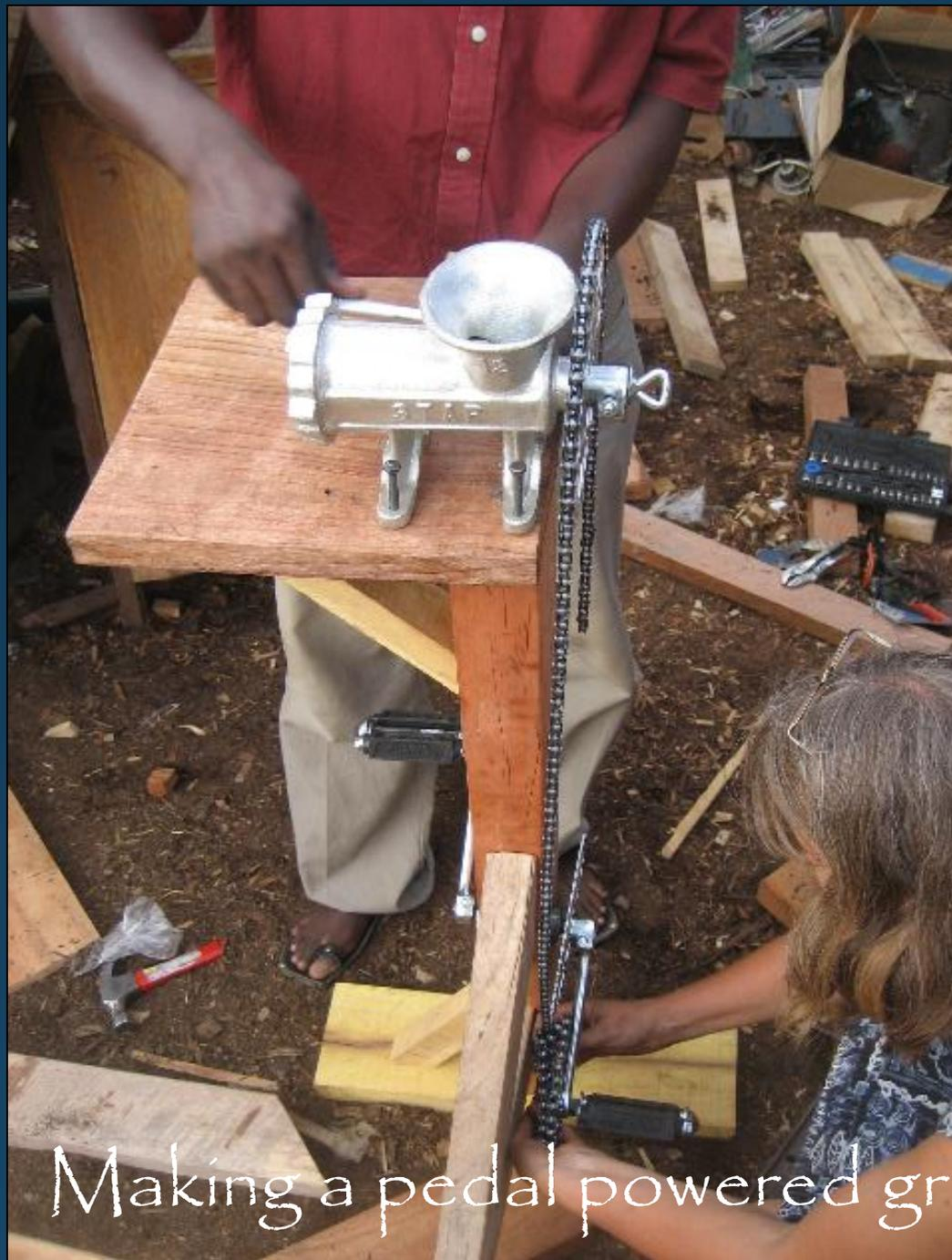
Making a pedal powered grinder
