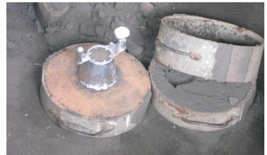
*A cast corn sheller with sprues attached.*
