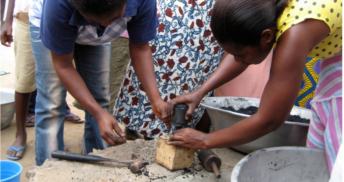
This project is a very low-cost device for forming charcoal briquettes. It is composed of three welded metal parts and a wooden block. To make it, you will learn to use a band saw, a sander, a drill press, the OMAX water jet cutter and several hand tools. You will also learn to do some basic welding.
