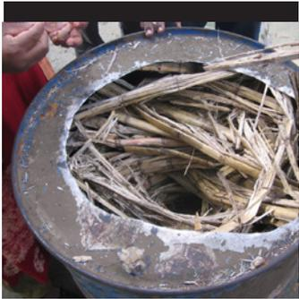
1. Placing bagasse in the oil drum
