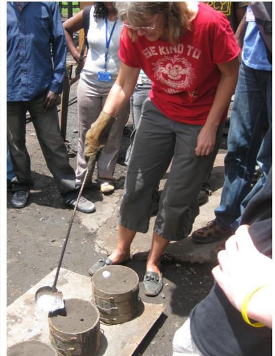
*Pouring molten metal into the molds.*
